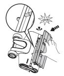
When replacing, always latch the brush cover into place to avoid leakage.
