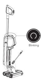
When the indicator of Dust Sensor Malfunction blinking, remove Dirty Water Tank, clean the dirt sensor with a damp cloth or the cleaning tool.
