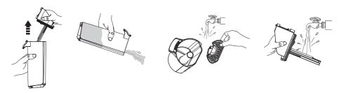
If the Dirty Water Tank lid and the filter inside have been blocked, remove the tank lid and the filter, rinse both parts with water.
